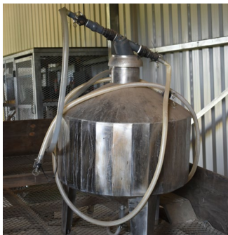
The piggy system that can help to apply herbicide or fertiliser.
